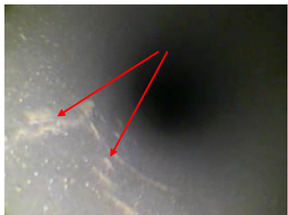
Pic 6: Tube 061-build-up of carbon and scabs
