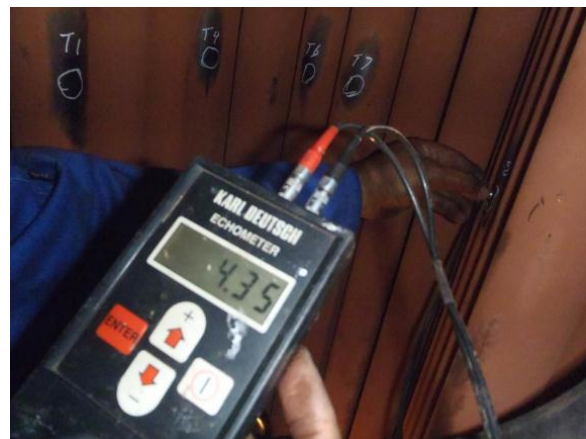
Pic no 1 & 2: UT reading of 6.86 @ the smoke tubes in Economizer No1. And 4.35 @ the smoke tubes in Economizer No 2.
