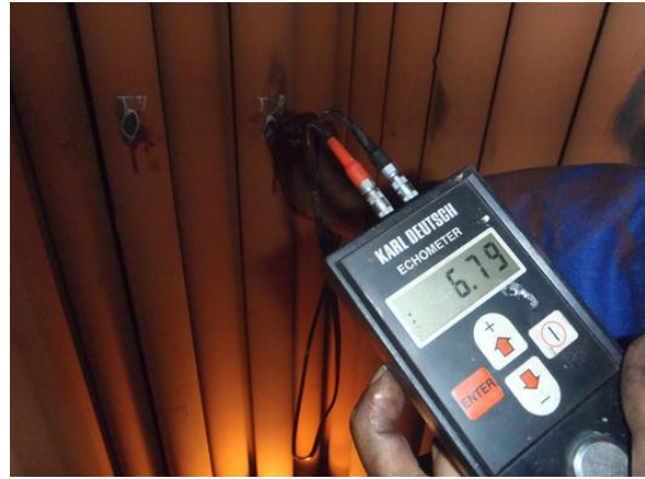
Pic 3 & 4: UT reading of 4.86 @ the smoke tubes in Economizer No 2. And 6.79 @ the smoke tubes in Economizer No 4.
