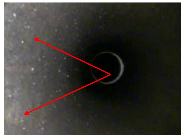
Pic 12: Tube 052- Soot and carbon build up con't
