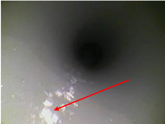
Pic 22: Tube 070- Scaling observed
