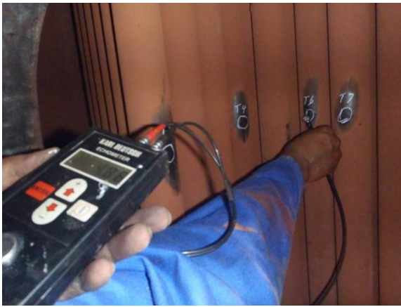
Pic 3 & 4: UT reading of 4.86 @ the smoke tubes in Economizer No 2. And 6.79 @ the smoke tubes in Economizer No 4.
