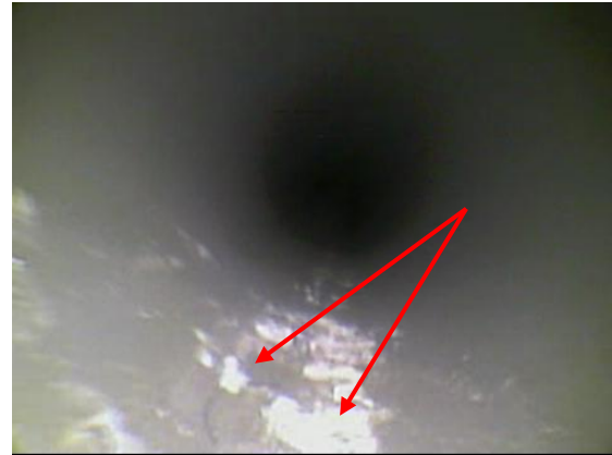
Pic 23: Tube 072- Scaling con't
