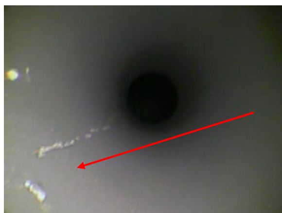
Pic 21: Tube062- Scales & soot observed
