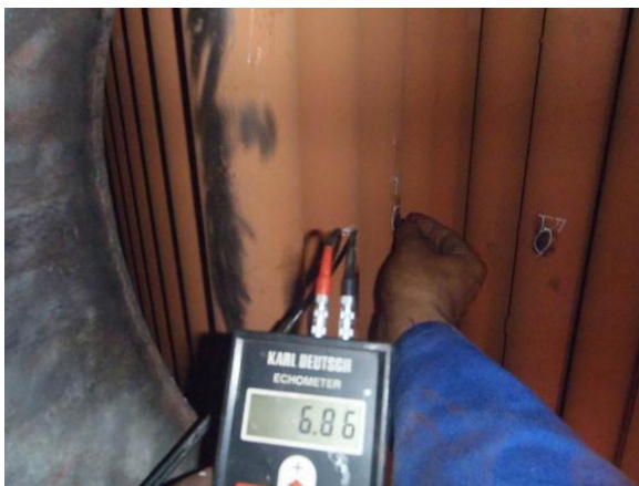
Pic no 1 & 2: UT reading of 6.86 @ the smoke tubes in Economizer No1. And 4.35 @ the smoke tubes in Economizer No 2.
