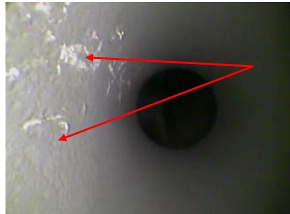
Pic 19: Tube044- Small amounts of scaling
